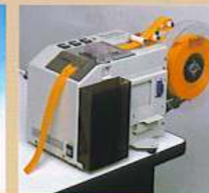
▲ UTP-III (TAPE PERFORATOR)
